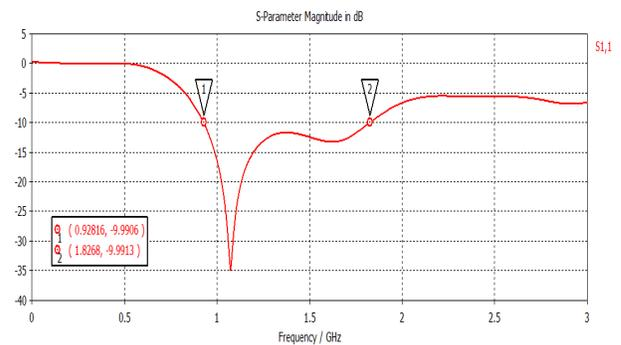
**Figure 2:** Simulated Result of the proposed RMPA.
