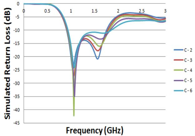
**Figure 4:** Simulated return loss of the proposed RMPA as a function of centre of semi-circle of the ground plane.
