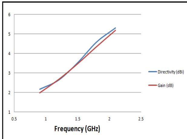
**Figure 3:** Directivity & Gain of the proposed RMPA in 0-3 GHz.
