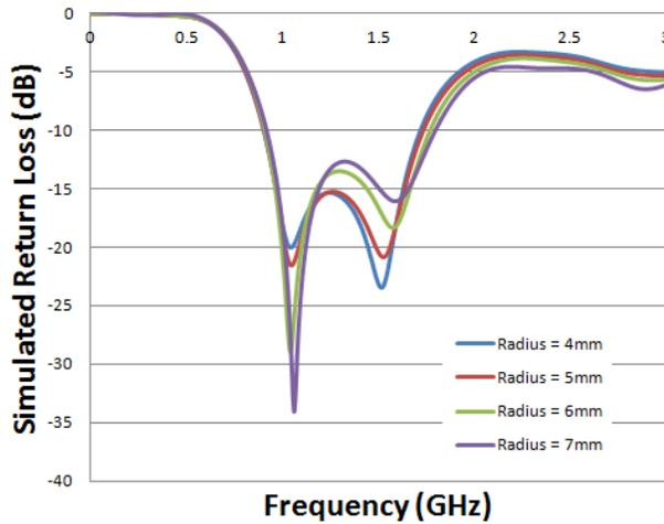
**Figure 5:** Simulated return loss of the proposed PRMA as a function of radius of semicircle ground plane.
