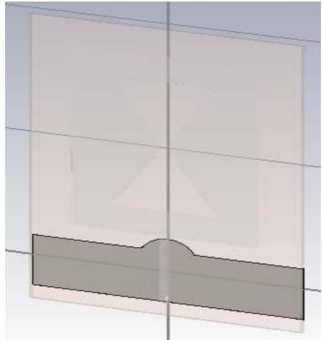
**Figure 1:** Structure of the RMPA with DAMRU shaped slot.
