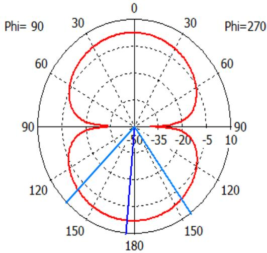
**Figure 3:** Simulated Polar View of Radiation Pattern Result of the proposed RMPA.
