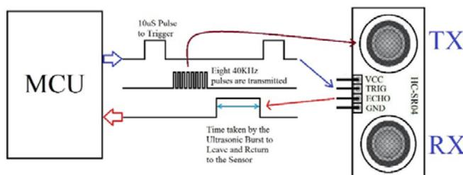
**Fig. 2:** Functioning of ultrasonic sensor module
